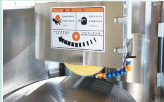
排水性とメンテナンス性に優れたステンレス製湿式カバー Stainless steel splash guard cover with excellent drainage and maintainability.
