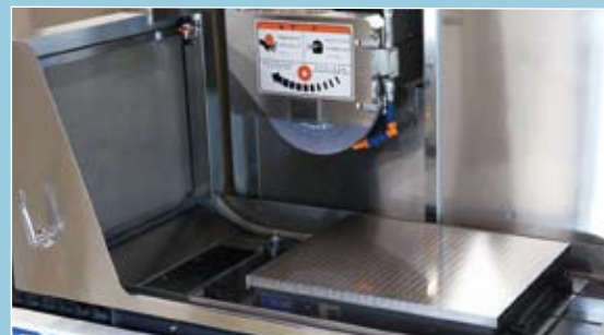
ワークの脱着が容易に行える広い開口部 Wide cover realized easy workpiece detaching.
